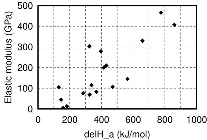
Figure 5.16: Plot of elastic modulus  $E$  versus heat of atomization  $\Delta H_a$  for a sample of mostly common metals.
