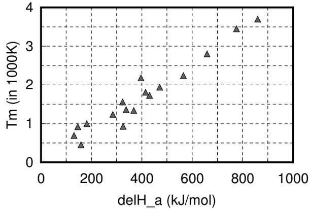
Figure 5.17: Plot of melting temperature  $T_m$  versus heat of atomization  $\Delta H_a$  for the same metals as in Fig. 5.16.
