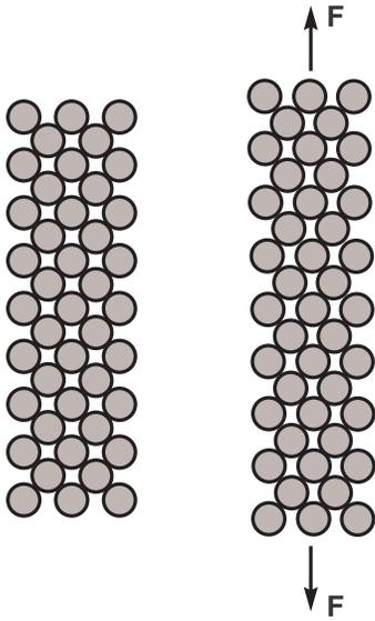
Figure 5.14: Atomic model of elastic deformation. Crystalline rod of FCC metal subject to load  $F$  in  $z$ -direction. Note axial stretching and lateral contraction.
